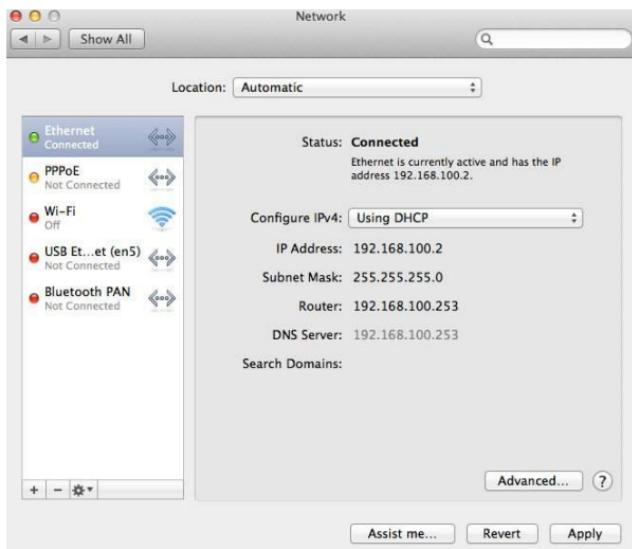
By default the automatic wired connection is Ethernet DHCP. If DHCP is enabled you can use this connection without IP address configuration. If DHCP is disabled, you have to configure the IP address manually.
